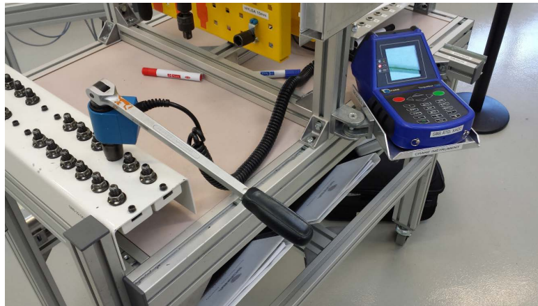
Figure 365: Applying and measuring torque (Image Roser)
