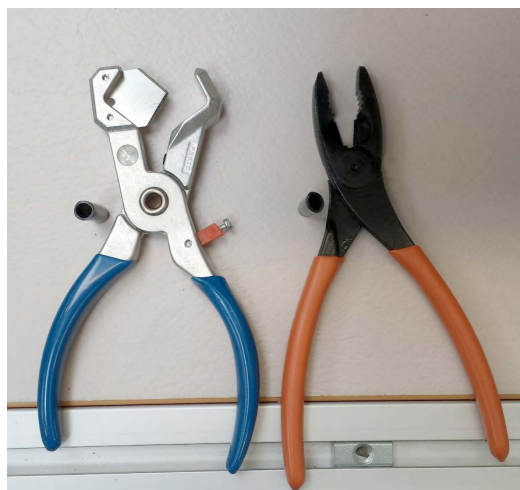
Figure 360: Good and bad pipe cutters (Image Roser)
