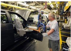
Figure 178: Car Seat Assembly (Image Ford Motor Co. under the CC-BY-SA 2.0 license)
