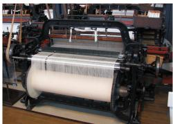
Figure 81: Toyoda Model G Automatic Loom (Image Roser)
