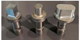
Figure 311: Selection of standard punch shapes (Image Roser)
