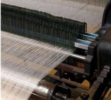
Figure 88: Toyoda Model G Automatic Loom Detail of Warp Break Stop (Image Roser)
