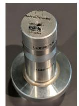
Figure 312: Trumpf Punching Tool Data Code (Image Roser)
