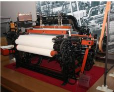
Figure 80: Toyoda Model G automatic Loom (Image Morio under the CC-BY-SA 3.0 license)
