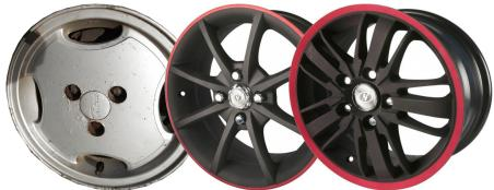
Figure 176: Three, four, and five lug nuts on a car wheel (Image Bindydad123 under the CC-BY-SA 4.0 license and (Image PXHere in public domain)
