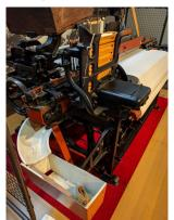
Figure 84: Toyoda Model G Automatic Loom Detail Automatic Shuttle Change (Image Roser)
