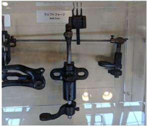
Figure 91: Parts for the weft fork (Image Roser)
