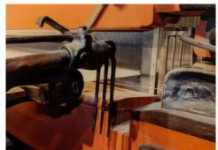
Figure 89: Toyoda Model G Weft Fork Mechanism (Image Toyota with permission)
