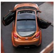
Figure 169: Hyundai Veloster, which has one door on the driver side and two on the passenger side (Image loubeat under the CC-BY 2.0 license)
