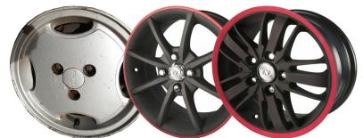
Figure 216: 3, 4, and 5 lug nuts (Image Bindydad123 under the CC-BY-SA 4.0 license and PXHere in public domain)
